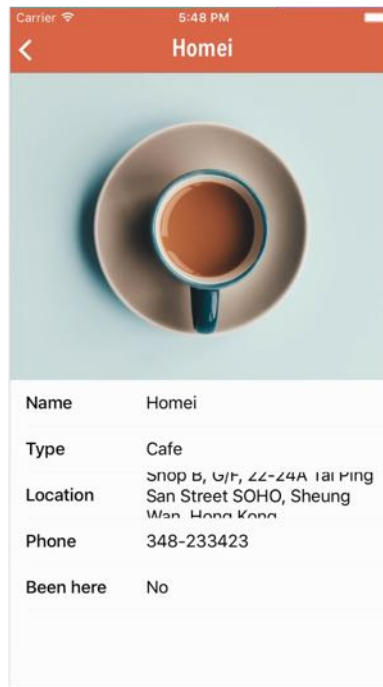
Figure 15-5. The location field is not correctly resized for address that takes up more than three rows
